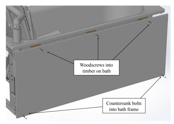
If **the bath is a detachable seat version, then follow this step.** If not, then move directly to Step 2. When there is a detachable seat present, it is important that the side panel which contains the pre-fixed magnets is fitted to the 'seat swing' side, as shown.
