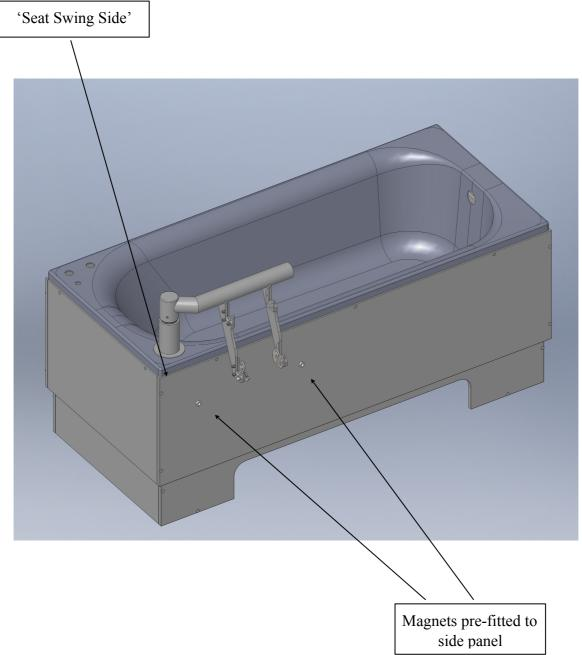
2. With the front panel fitted, the end panel(s) can be fitted. Firstly, these can be secured along one edge to the front panel using M6 x 40 countersunk bolts, which screw through the front panel into the threaded inserts located in the holes in the sides of the end panels. As these bolts are tightened ensure that the end of the front panel is flush with the face of the end panel, and that the top faces are also aligned. The bolts are finished off with a white cap.
